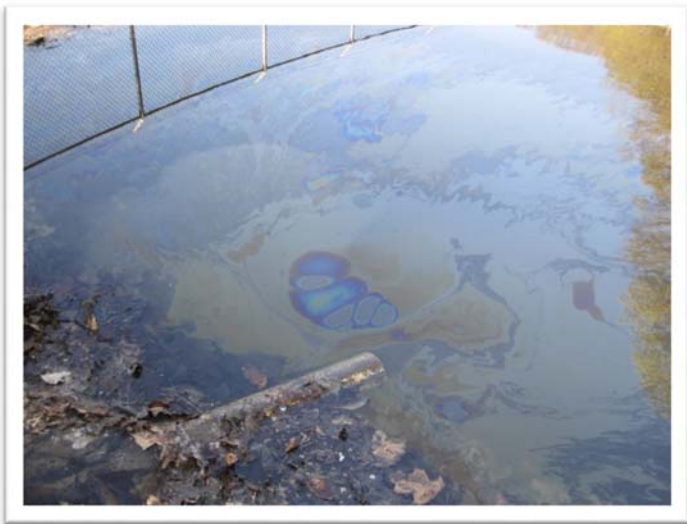
When disturbed, an organic sheen will crack and break into many small platelets.
