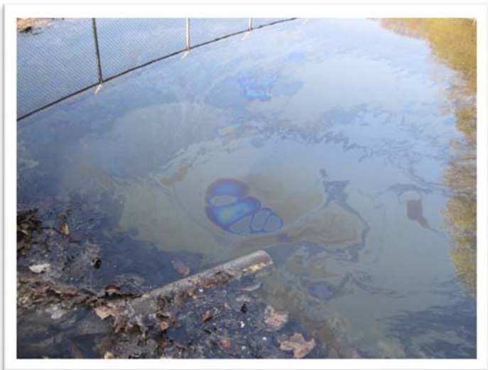
When disturbed, an organic sheen will crack and break into many small platelets.
